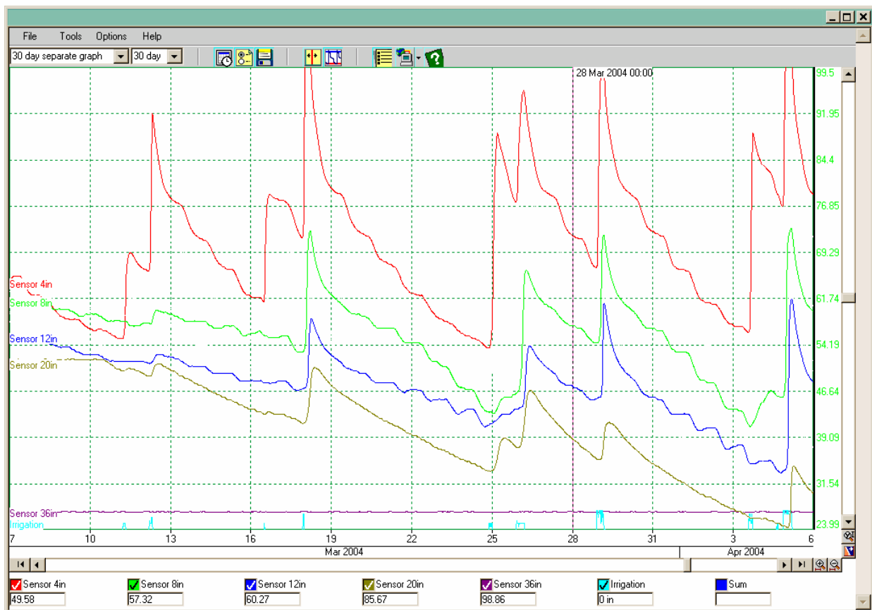
Fig. 1. Separate layer graph showing root activity (stepping) down to 12 inches in depth. Note no “stepping” at 20 inches indicating no root activity at that level.
